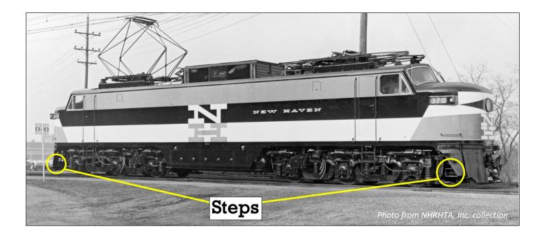
The Rapido HO scale model of the EP-5 includes these steps, but they were not installed at the factory for a very good reason; if installed, they prevent the shell from coming off the chassis without removing the steps first. Therefore...
