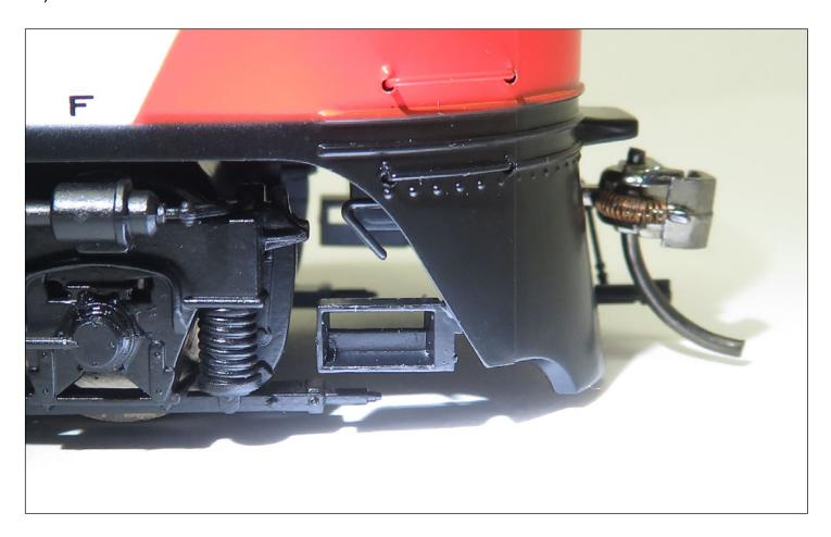
7). If you need to remove the shell to gain interior access to the EP-5 after the steps have been applied, simply twist gently on each step to break the (hopefully) weak glue bond. With white glue, it won't take much force. If you used a permanent adhesive and you want to remove the shell, we're sorry but your steps are going to get broken (we did warn you!).
