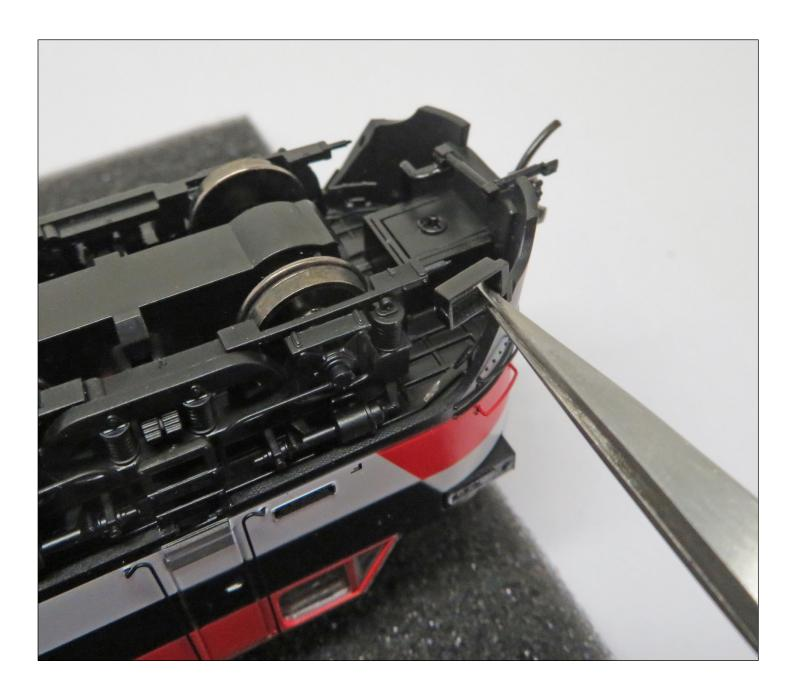
5). Before the glue sets, orientate each step so it is parallel and in line with the track as seen in the red ovals in the photo. Note how the steps are now out over the chassis, which prevents the shell from being removed with the steps installed.
