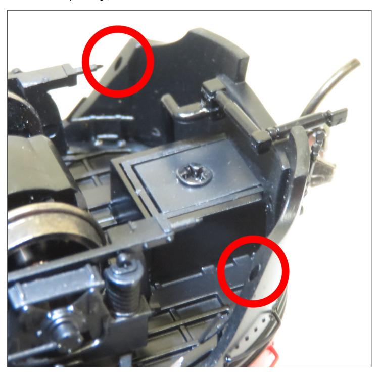
3). The steps can be identified left and right by looking at the open side of the step and the mounting peg's location. The open side of the step box should always face outward on the model and the mounting peg should be closest to the nearby coupler.
